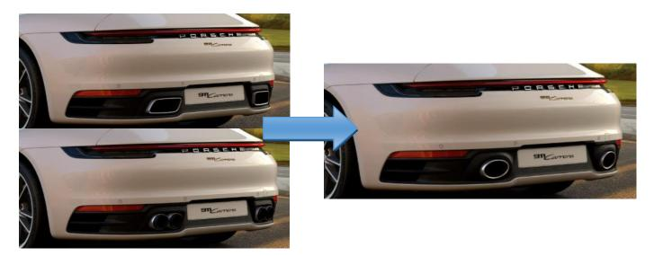
The following Porsche part numbers must be ordered according to the region where the car is located because different regions use different number plate dimensions and thus different diffuser part numbers.
