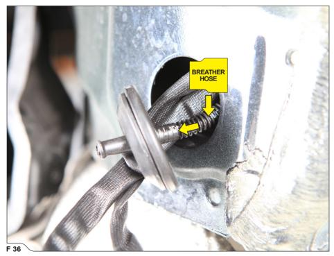
IMPORTANT: make sure, you plug the battery breather hose into the grommet, as shown!
