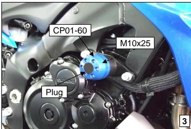
**The assembly is shown at the right side, the process are on the left side principle the same!**
