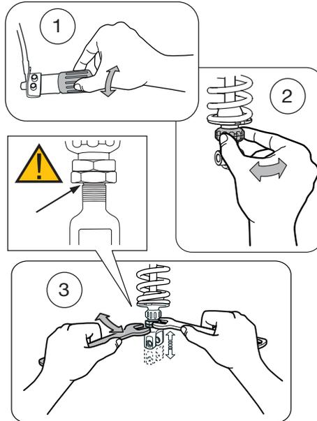
upper nut with one hand and at the same time loosen the lock nut (lower nut). Turn the end eye/ bracket to the desired length. Lock the lock nut. Tightening torque: 40 Nm
