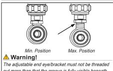
out more than that the groove is fully visible beneath the lock nut. This is maximum length. After adjusting, make sure that the lock nut is tightened (30Nm).
