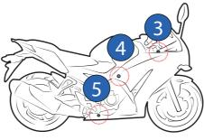
8 Remove the center fairings on both sides by loosening the eight screws (1)(2)(3)(4)(5)(6)(7) (8).
