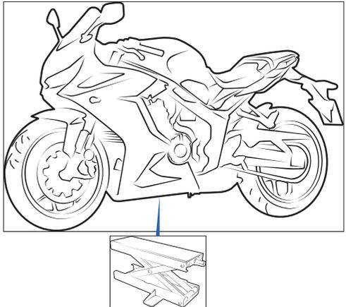
2. Loosen the screws ①② on right side and ③④ on left side in order to remove the chainguard and mudguard (A).
