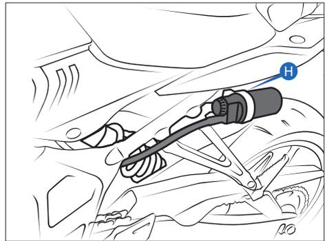
6.5 Right side, Install the sleeve (thickness 5.5mm) position between the rear sub-frame and the foot peg by using the screw M8x35
