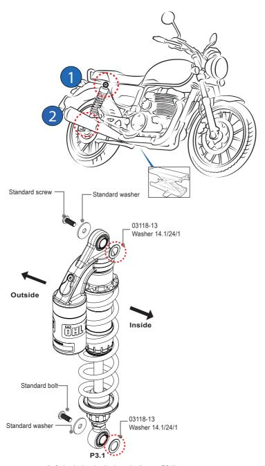
(Left shock absorber is shown in diagram P3.1)
