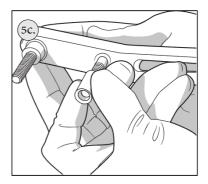
d. Clock the reservoir in the reservoir bracket so that the head of the banjo bolt is oriented towards the damper, and that the clamping surface on the reservoir is centered in the clamp, then tighten the pinch bolt to finish installation on this side.
